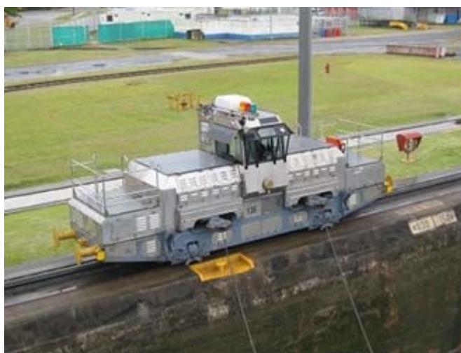
Electric locomotive (mule) used in original locks
